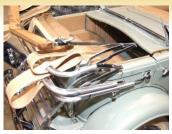
The complicated convertible top mechanism is shown in the lowered position before the canvas top material was installed.
