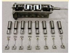
Inside the straight eight engine are all the correct parts custom machined to scale from steel, cast iron and aluminum.
